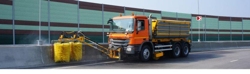
Street sweepers are used for cleaning solid coatings of transport infrastructure facilities. The operational work of the street sweeper consists of sweeping the surface, collecting the dust into the storage container, transporting it to the waste burial site and emptying the storage container there. Then the operation cycle is repeated.
