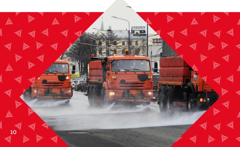
During the rain, the dust, which has gotten in between the asphalt particles, becomes wet, and therefore it is easier to wash it away. By doing so we use water sparingly. The street sprinkler has to only direct a strong stream of water at the slushy dust. As a result, roads become cleaner quicker. Rain can only lay the dust while the street sprinkler washes and cleans it away from the streets.
