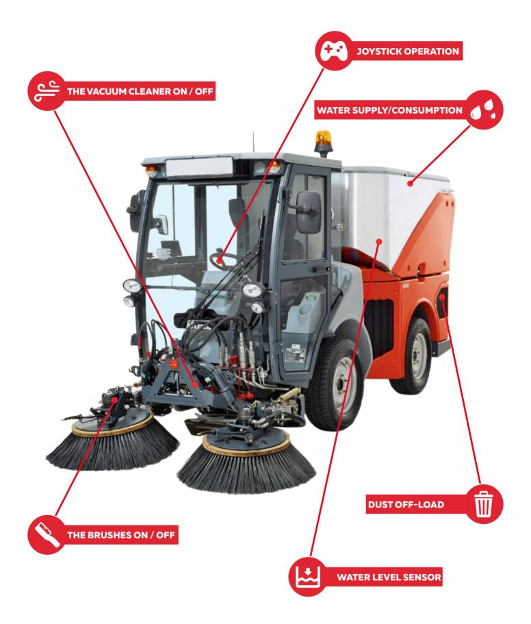
Street vacuum sweeping vehicles «V-Sweepers» are used to clean streets in large cities from dust, small debris, stones commonly found on the roadway and load all this stuff into the receiver hopper.
