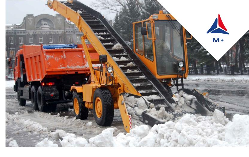
Clearing of formed snowballs and swept snow is also performed by snow-removing vehicles equipped with a screw conveyor (a working rotating tool). The vehicles move away snow packs and perform their direct discharge at a remote from the roadway distance.
