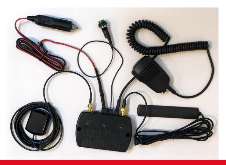
GPS/GLONASS/GSM terminal provides the determination the vehicle location and telemetry indicators (speed, route, parking lots, fuel level, «ignition», emergency two-way communication) and the transmission of this information to the processing server using GPRS channel. All data not transferred to the server is stored in non-volatile flash memory, which allows to use the terminal as a «Black box», with their data transferred to the server when the communication channel is recovered.
